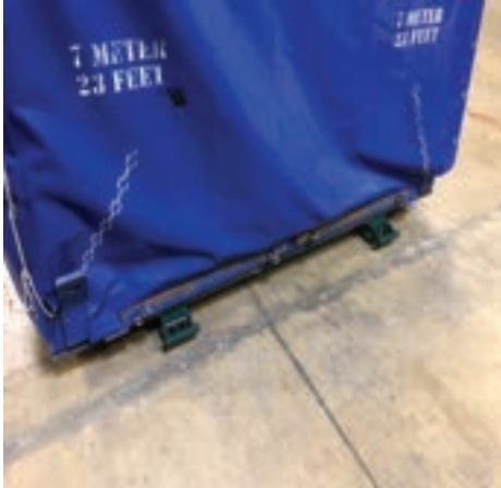
Placing the dollies where support is needed ensures the rear dollies will be kept parallel in order to track properly when moving.
