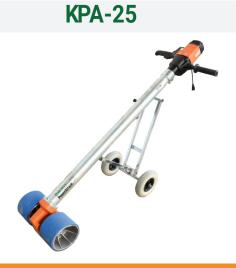
**Corded-25 Ton Capacity** Powered by an electric cable either with 110V or 230V (KPA-25-230V) drive motor
